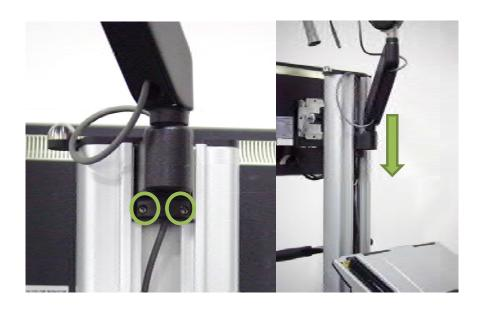
Reinstall small channel cover number 4 above camera arm.
